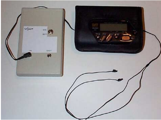
Figure 2: The used portable Sony TCD-D8 DAT recorder coupled with Sennheisser microphone capsules
